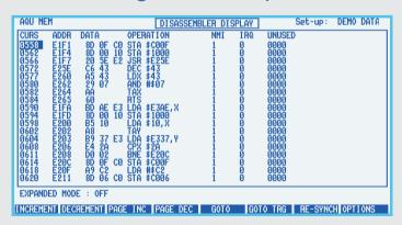
Disassembler pods with built-in firmware are available for a wide range of popular 8-bit and 16-bit microprocessors. Because the disassembler firmware is incorporated in the pod, disassemblers can be interchanged at will.
